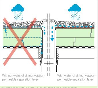
Inverted roof with double-layer insulation and gravel layer
